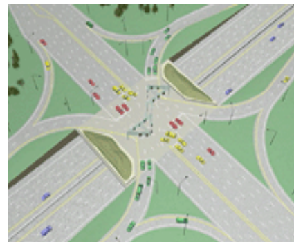
Figure 1 Typical Layout Single-point Urban Interchange
