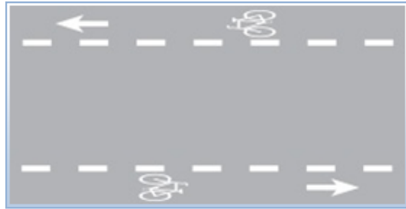
Typical Striping for Bike Lane on Roadway
