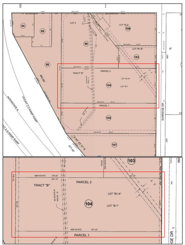
Dashed lines represent easements for a sewer line and a gas line.
