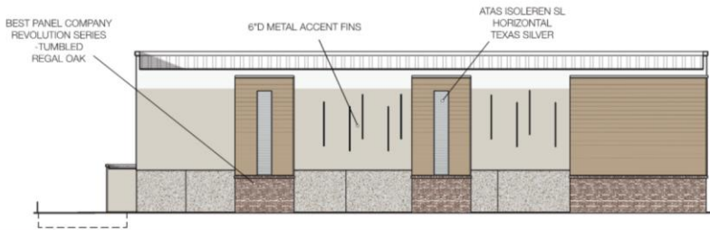
NORTH ELEVATION: BUILDING B Scale: 1/16" = 1'
