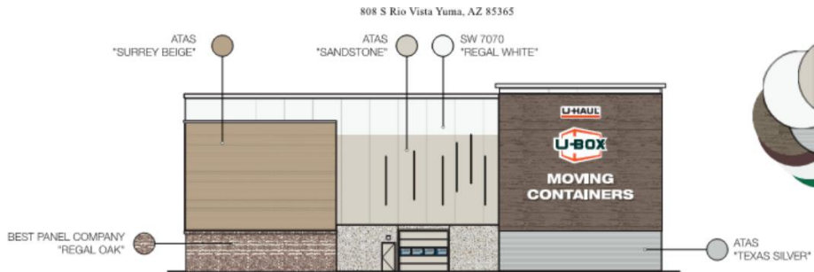
WEST ELEVATION: BUILDING B Scale: 1/16" = 1'
