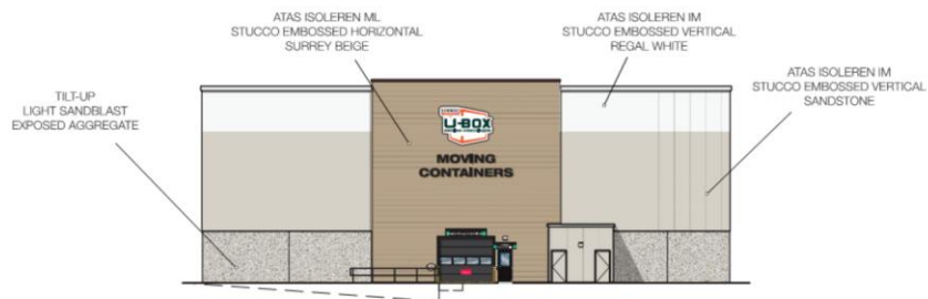
EAST ELEVATION: BUILDING B Scale: 1/16" = 1'
