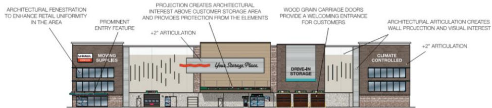
NORTH ELEVATION: BUILDING A Scale: 1" = 2'
