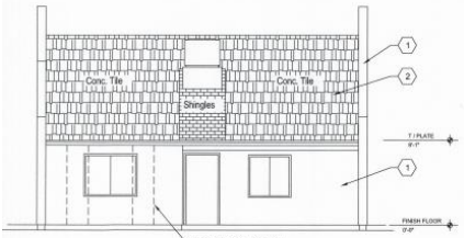
1 Rear Elevation SCALE: 3/16"=1'-0"
